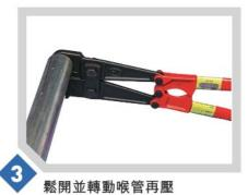
Release and rotate pipe for second dot
